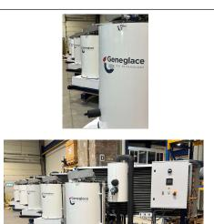
The production of the 5 Geneglace ice machines type PACK 32 is finished. These PACKS with a daily production of 26 tons per day (with water at 25°C and air at 35°C), will be associated with 5 manual compactors. Beginning of November, they will be shipped in containers to Africa..
